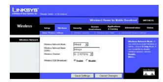
Figure 8-18: Wireless Tab - Basic Wireless Settings
